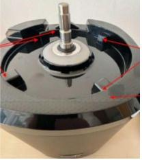
90. These means prevent the housing from rotating and moving sideways and falling off the drive unit when in use and therefore fix the housing to the drive unit according to feature [1N]. As discussed, it is of no relevance that the fixation does not prevent the housing from being vertically lifted and vibrating.
